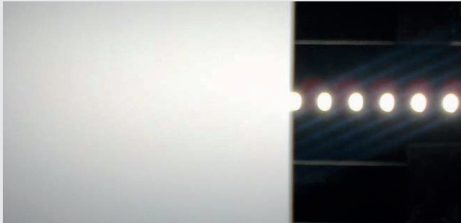
Fig. 3: Light channel with LEDs spaced at 8 mm. Cover spaced at 10 mm.
